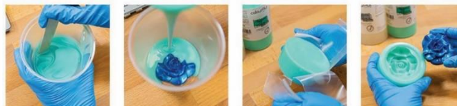
Mix Part A/B evenly Pour the mixture into mother mold with outflame Wait for 6-8 hours to demold Take out the moth mold from silicone mold
